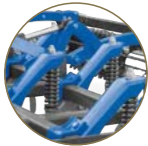
Safe and vibrant work with independent springs
