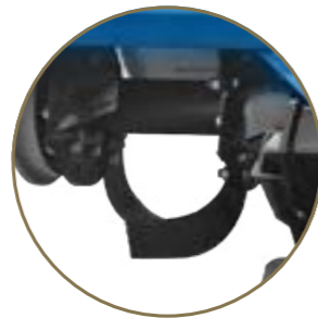
Hydraulic sliding system ensuring safety for trees
