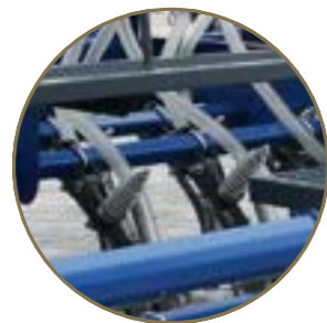
Spring tines offers machine safety
