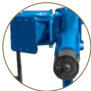
Mechanical and hydraulic adjustment of working-width
