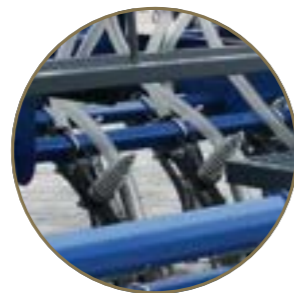
Spring tines offers machine safety
