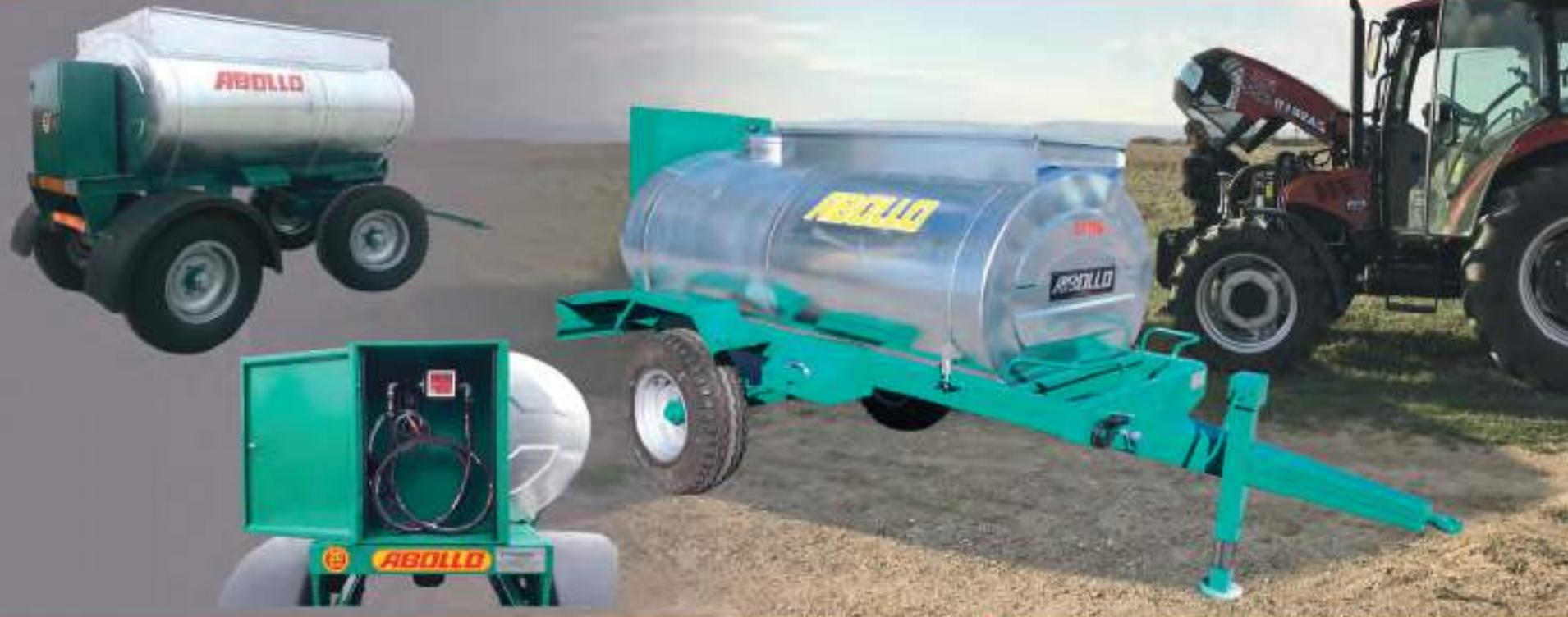
The ABOLLO FUEL TANKER is produced in two different types as single axle and double axle. The tank is galvanized stainless steel and does not suffer corrosion. Thanks to the fuel filling system located inside the cabin, the desired fuel amount is transferred from the meter.
