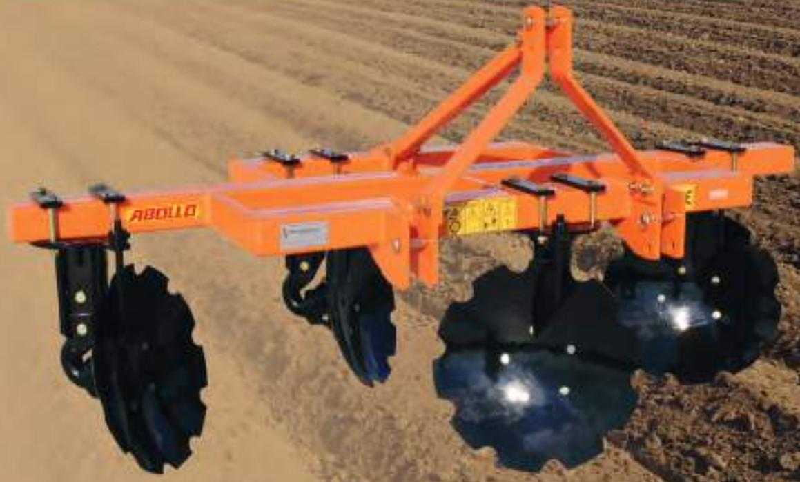
The ABOLLO DISC FURROWER is used in the mechanized building of a solid furrow or ridge of 30 to 35 cm in height and adjustable width in accordance with the recommended spacing for the crop, preparing for the planting and / or performing the so-called "ridging", which consists of placing soil on the roots of crops (potato, sweet potato, cassava, yam) and others such as tobacco, peanuts, pineapple etc.. This operation is vital to the management of weeds and formation of the root system.
