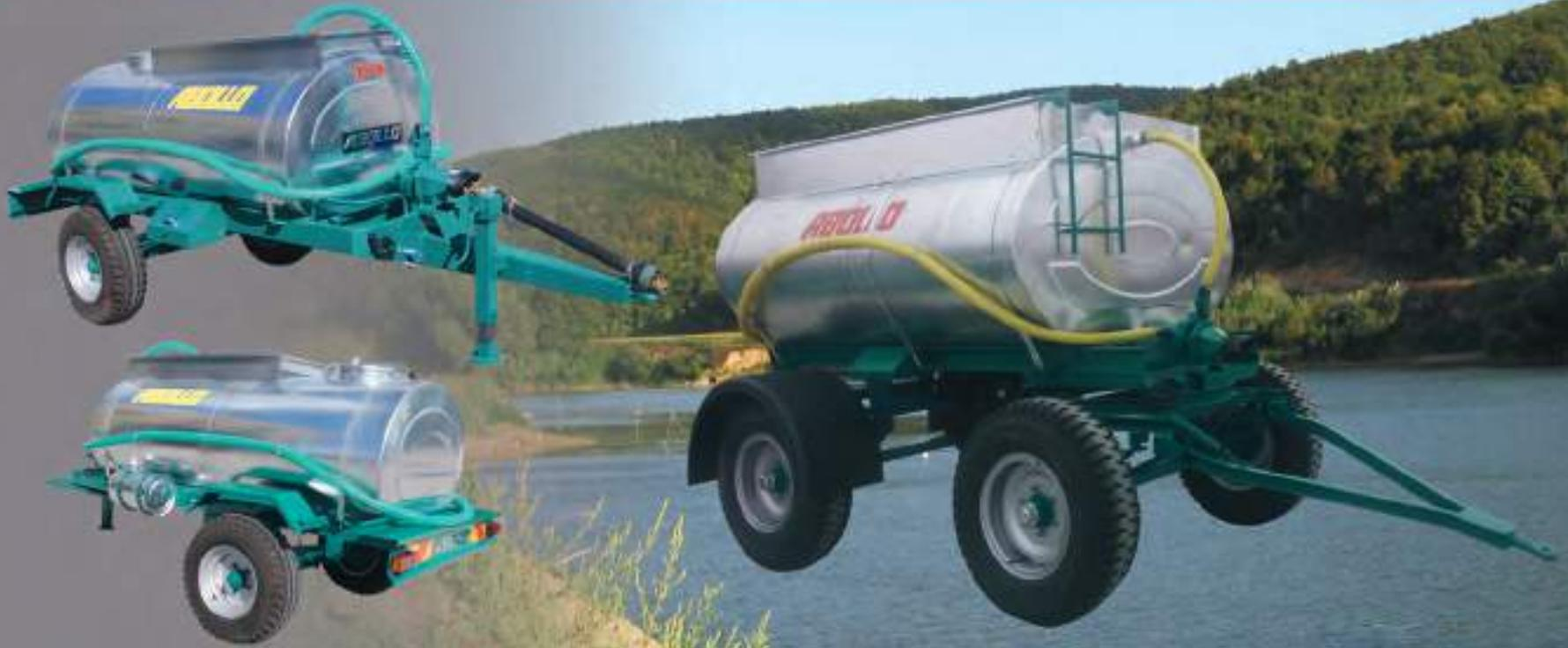
The ABOLLO WATER TANKER is produced in two different types as single axle and double axle. The centrifugal pump is started by the action taken from the tractor pto shaft. Pump 2 with "inlet and 2" outlet is used for filling and emptying the tankers behind the tractor. Thanks to the self-filling system, the water tank is filled with the pump. Thanks to the special oil in the pump, high cycle heating problem is prevented. The tank is galvanized stainless steel and does not suffer corrosion.
